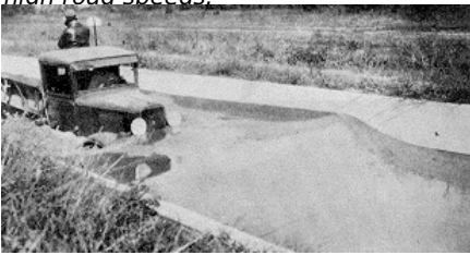
A light truck undergoes the water course during cross-country mobility tests, in 1935, at the automotive laboratory, Aberdeen Proving Ground, MD. The course consists of a concrete tank 250 feet long by 15 feet wide by 4 feet deep.
